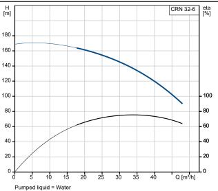
Pumped liquid = Water Liquid temperature during operation = 20 °C Density = 998.2 kg/m³
