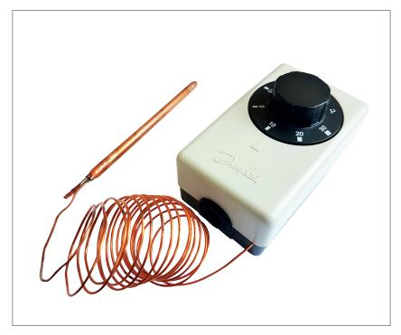
The UT thermostat is a temperature-controlled electric switch with copper capillary and sensor. The temperature can be set easily and accurately using the large knob on the front of the thermostat. The temperature must be set to correspond to the required mean temperature.
